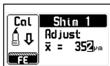
Figure 2.8: Shim calibration thickness adjustment screen
