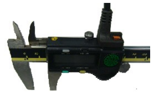
Interface Cable for Mitutoyo Caliper model 500-171-20B
