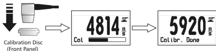
Figure 2.4: Zero calibration procedure
