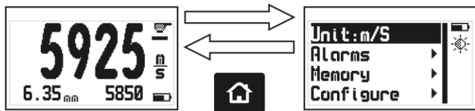
Figure 3.2: The “Home” key from the measuring screen
