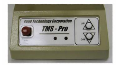
Basic control of crosshead movement is possible from the test stand itself.
