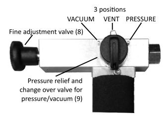
Turn the fine adjustment valve (8) counterclockwise fully out (smooth "stop" can be felt).
