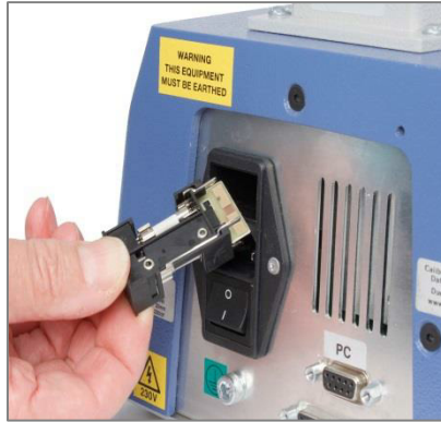
Carrier removed to replace fuse
