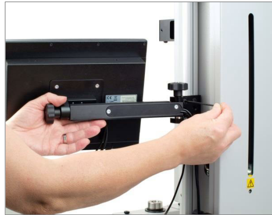
Fix the upper Torx screw first
