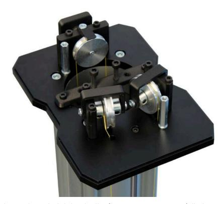
In the image above, the left-hand pulley (lower extensometer arm) displays a typical fault that can occur when the device is improperly handled.
