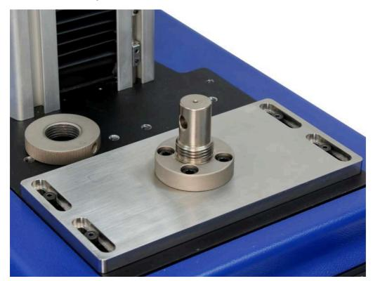
Using the QC fittings secured to the anvil plate and ELS, ensure that the test setup is aligned by lowering the crosshead of the test stand so that the position of both the upper and lower QC fittings can be compared against each other.
