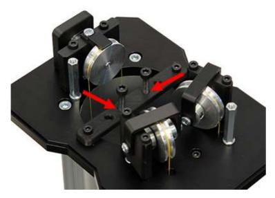
To ensure the screws remain with the device they should be screwed into the two threaded inner holes in the counterweight transit mechanism, as shown in the image above. When securing the screws ensure that they do not interfere with the travel of the counterweight.
