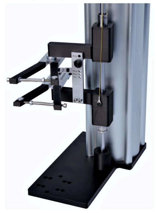
As standard, the MLTE gauge setting plate offers four set gauge lengths, plus one calibration point: 20 mm, 25 mm, 40 mm and 50 mm.
