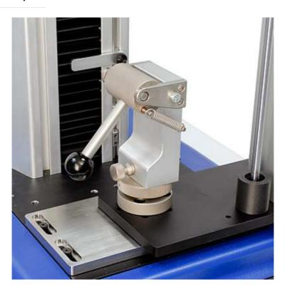
Once the QC adjustment ring is in place, fit the grip on top of the post and secure the retaining pin. As shown in the image above.
