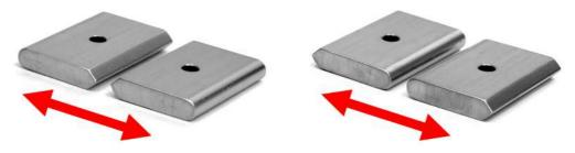
To provide maximum specimen shape compatibility, the extensometer is supplied with double-sided knife edges that feature two different grip faces:
