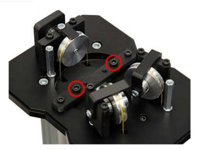
Using a **Hex key,** remove the two caphead screws located in the counterweight transit mechanism (highlighted above). Each screw should be undone in an **anticlockwise** direction.
