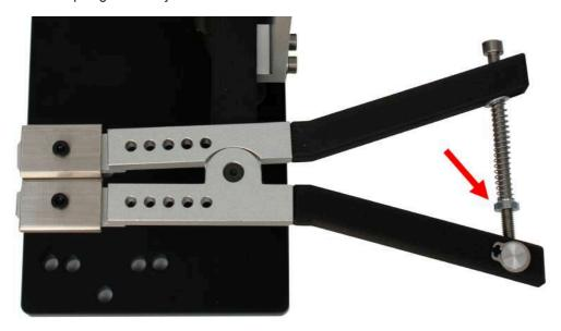
The thumbwheel location is shown in the image above. Turning the thumbwheel clockwise increased the gripping force while an anticlockwise movement reduces the force.
