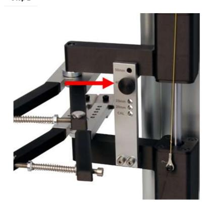
In this example, a gauge length of **'40 mm'** is required. Insert the gauge length setting pin into the hole identified as '**40mm'** on the gauge setting plate, as shown in the image above.
