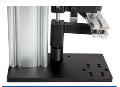
With the MLTE on a stable surface, rotate the MLTE so that the longest side of the base plate runs from left to right across the test stand. As shown in the image above (the front of the test stand is represented by the blue line). Ensure safe handling procedures are followed when lifting the device.
