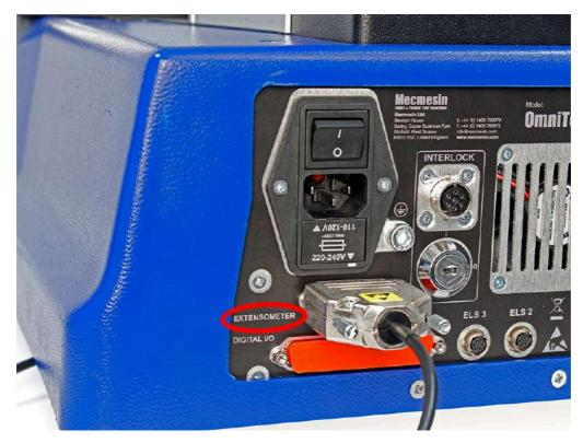
MLTE devices connect to Mecmesin test stands using a 15-way D-Sub connector:
