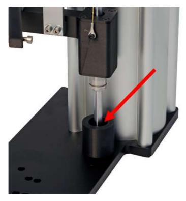
During transit, the lower extensometer arm is secured in a bearing cup at the base of the MLTE (highlighted above). To remove the arm from the cup, first move the upper arm to the top half of its travel. This ensures the upper extensometer arm is not impacted when releasing the lower arm.
