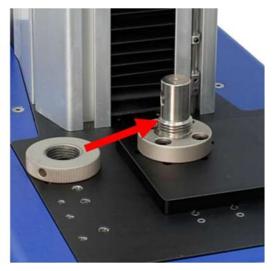
Before attaching the grips to the MLTE ensure the QC adjustment ring is fitted to the QC post, as shown in the image above.
