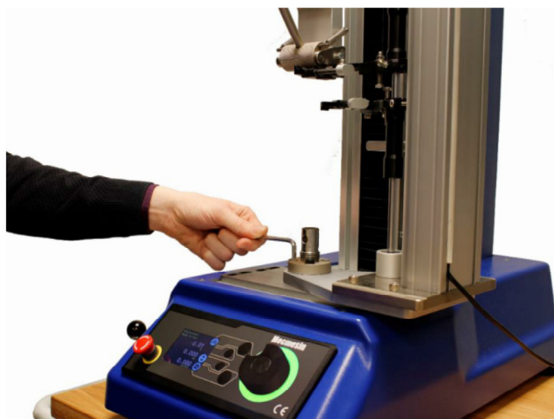
▲ Using a 4mm Allen key to secure the QC fitting
