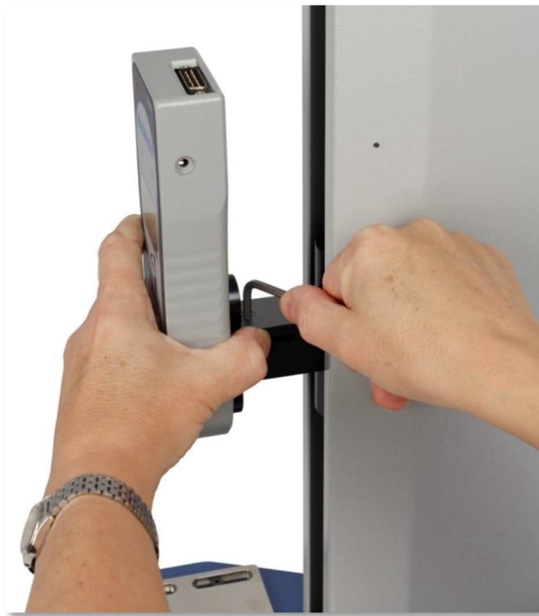
▲ Tightening the dovetail when mounting the force gauge
