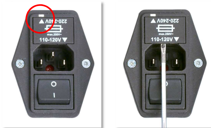
▲ Removing the fuse holder
