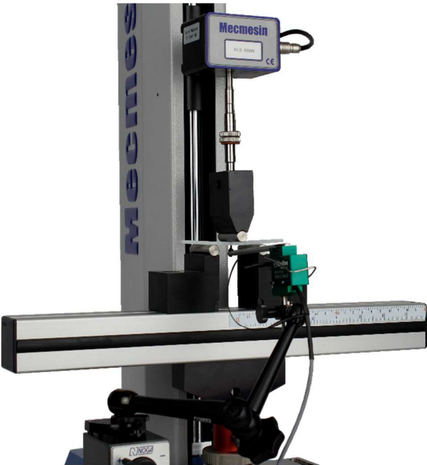
▲ A MultiTest- dV 2.5kN in dV(u) mode performing a 3-point bend, using an ELS 500N and deflectometer
