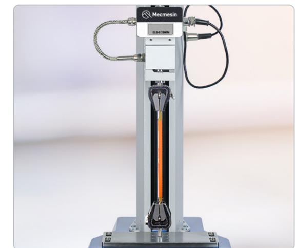
▲ Tensile strength measurement of plastic tubing
