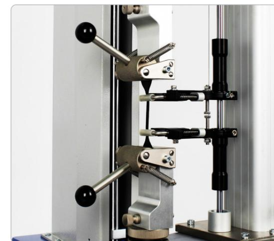
▲ Stress/strain measurement on rubber dumbbell specimen
