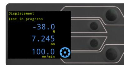
▲ Colour display of speed, displacement and load
