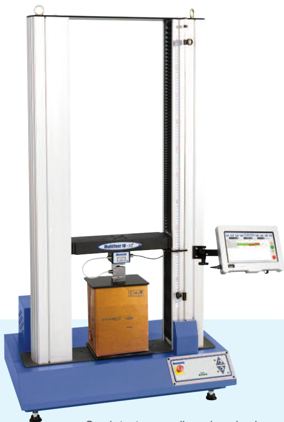
Crush test on cardboard packaging using a MultiTest 10-xt Top-load tester
