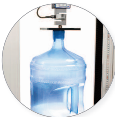
Top-load test on a water-cooler bottle
