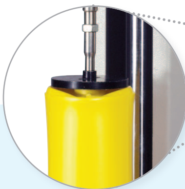
Top-load test on a water-cooler bottle
