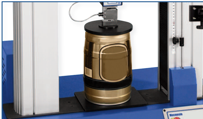
Top-load test using a circular compression plate
