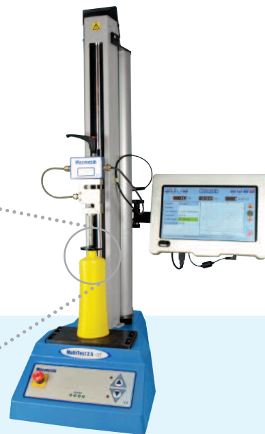
Top-load test on a PET bottle using a MultiTest 2.5-xt Top-load Tester
