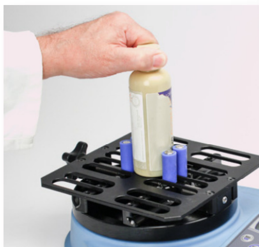
▲ Testing release torque of plastic closure using Tornado manual tester
