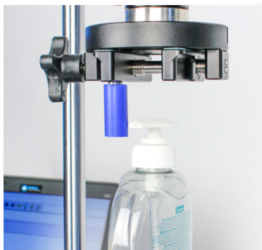
▲ Testing opening torque of closure/dispenser using Vortex automated tester
