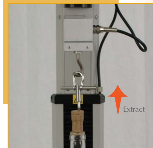
System converted to cork extraction tester
