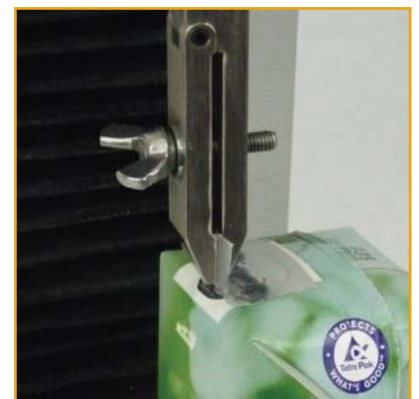
Peel test of induction-sealed foil tab
