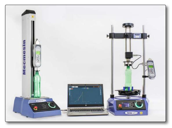
For some tests with Mecmesin digital instruments, plotting force or torque against time reveals essential sample characteristics, even though a displacement or angle axis is not possible. By connecting these devices to a PC with VectorPro Lite, you add live graphing and standardised calculations for immediate examination, comparison and analysis, and print or save reports with test annotations.
