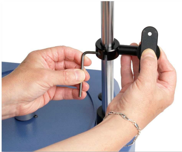
▲ Fitting the AFTI bracket using a 4mm Allen key
