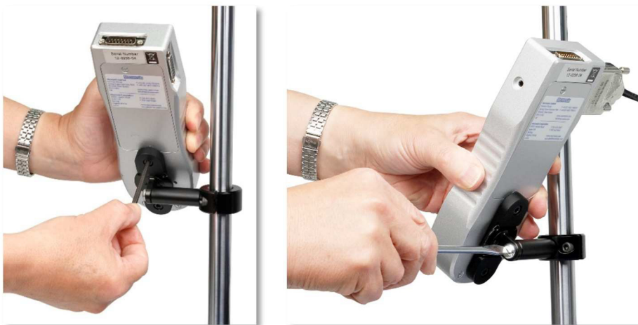
▲ The left-hand image shows the AFTI being secured to the bracket, while the image on the right shows how to adjust the angle of the AFTI.
