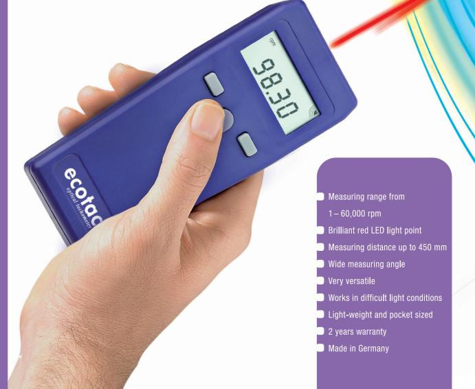
**The ecotach measuring principle**. The red LED light beam is reflected by a reflection mark fixed on the equipment to be measured. Observe the On Target indicator in the display to ensure accurate readings and read off the result from up to 450 mm distance and at a very wide angle. The device is very resistant to extraneous light, thanks to the use of an very bright LED and matching optical system.
