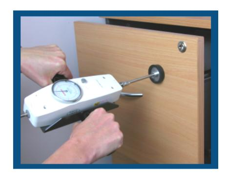
The Analogue Manual Handling Kit is a cost-effective solution to Occupational Health and Safety force testing applications. The Analogue Manual Handling kit can also be used to test isometric muscle strength or ergonomic applications such as accessibility for wheelchairs, walkers and those with limited strength capabilities, suitability of handles, grips and switches, and effectiveness and safety of household aids and assistive devices.
