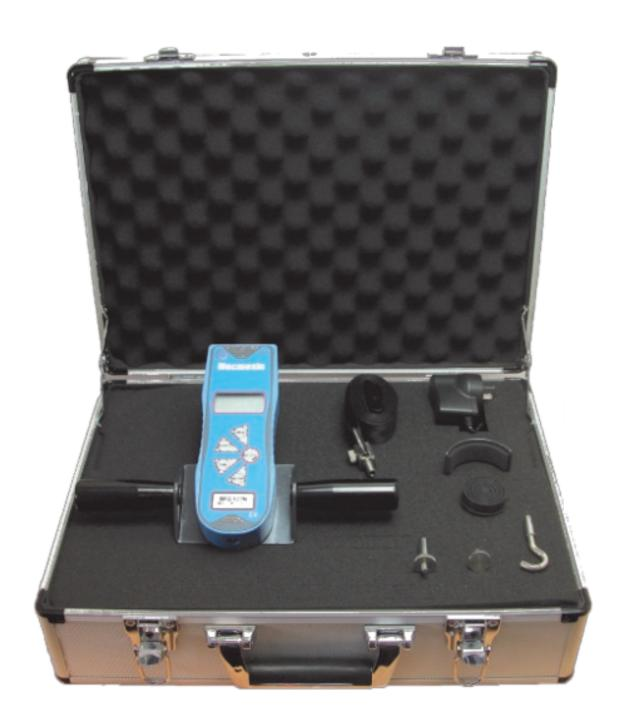
The Digital Manual Handling kit consists of a digital force gauge plus appropriate accessories to accurately assess each task application by mimicking the persons action. This kit is designed to not only measure the force used in physically demanding tasks, but also the capacity of personnel to perform operational tasks which require personnel to exert physical force to push, pull, lift, carry or use repetitive rotational movements day-to-day.
