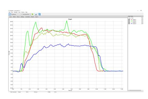
Use in conjunction with EasyPlot graphing software to plot the amount of force in real time. The software is invaluable where it is helpful or necessary to know the progress of force over a given period of time. Multiple tests are easily compared.
