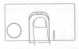
2). Push the golden metal chip outside to make the cell bounce up; with small tweezers, remove the exhausted cell. See below:
