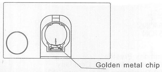
3). Insert the new cell below the golden metal chip with the + marking up, and then press it down to fasten. See below:
