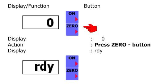
If rdy is displayed, the device is ready for recording data.
