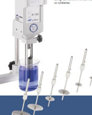
Measurement systems. A wide range of measurement systems allows the accurate determination of viscosity over an extensive range of products. The measuring systems are manufactured according to DIN 53019 for standardized determination of absolute viscosity - this creating the conditions for optimal comparability of viscosity. Measuring systems designed according ISO 2555 and Cone & Plate systems are available.
